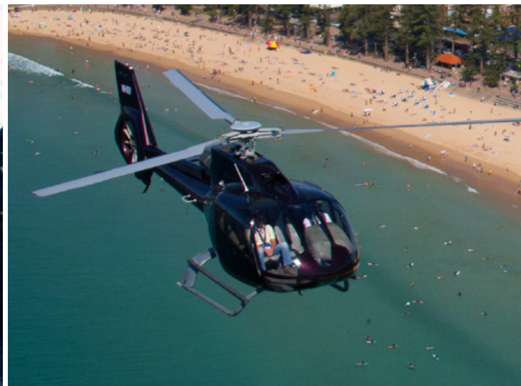
The Eurocopter EC130 is a single engine turbine helicopter manufactured in France. The EC130 includes all the latest technology, has a cruise speed of 115kts and has a very spacious cabin that can accommodate pilot and 6 passengers all with forward facing seats.
