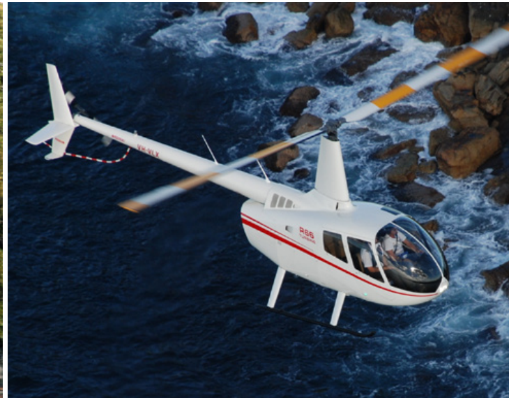
The Robinson R66 is a single engine turbine helicopter manufactured in the USA. The R66 can accommodate pilot plus 4 passengers and has a cruise speed of 110kts.
