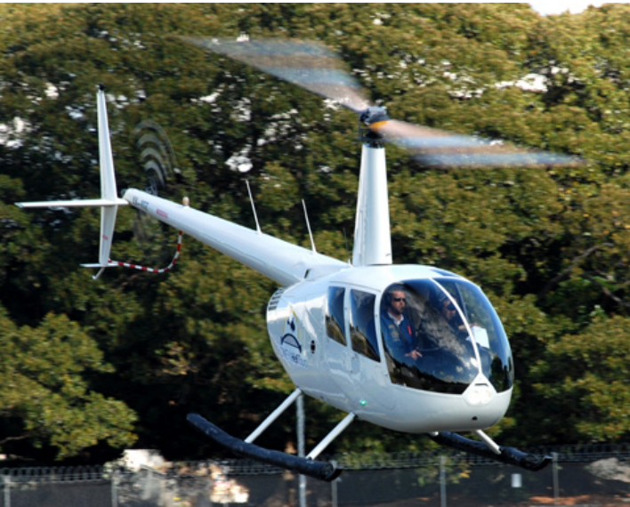
The Robinson R44 is a single engine piston helicopter manufactured in the USA. The R44 can accommodate pilot plus 3 passengers and has a cruise speed of 100kts.
